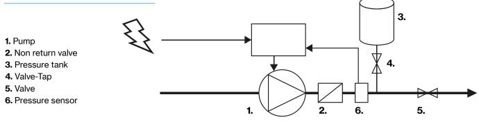
Pressure tank volume suggested: 10% of the capacity of the system
