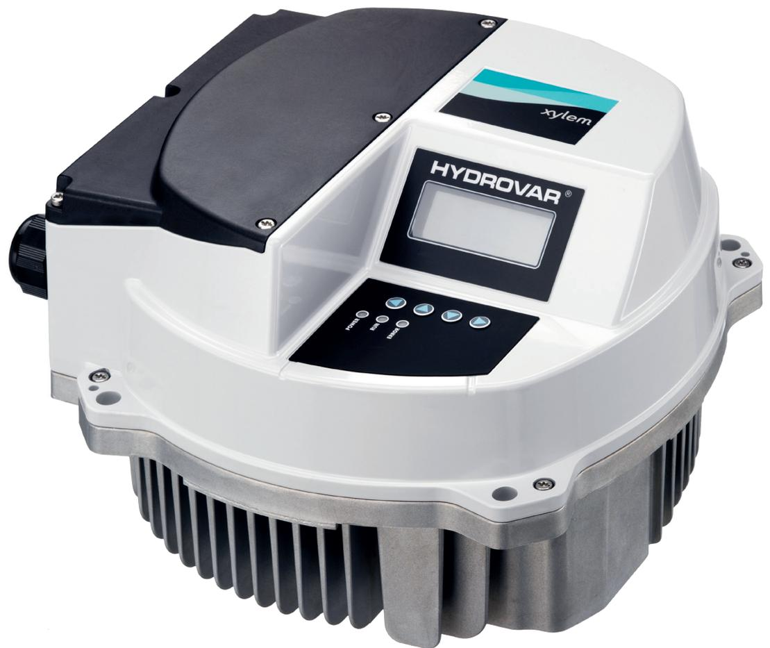
Retrofitting the 'plug and play' HYDROVAR units to a fixed speed booster set not only eliminates the need for a control panel but also introduces a soft start function, that when combined with the benefits of running a pump at a variable speed, can prolong the life of the pump and the water system. By reducing the in-rush current when the pump is turned on, parts such as motor bearings and pipe fittings are protected from hydraulic shock that can cause cavitation and breakdown.
