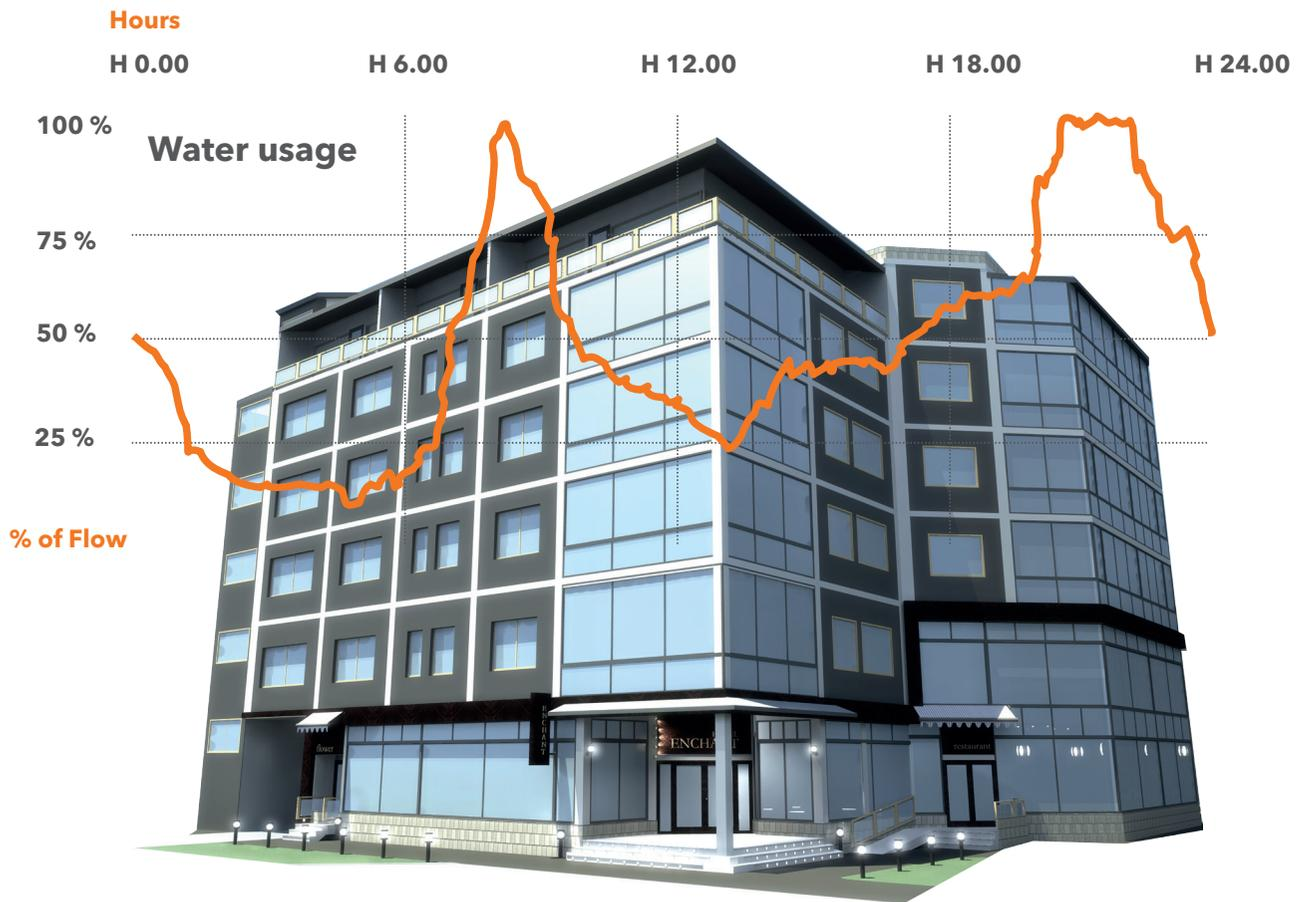
Water consumption in a hotel is not uniform during the day. The pumping system should be able to match the real needs of the users.
