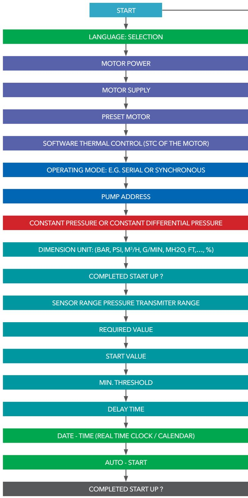
AFTER 10 MINUTES IF THE START UP IS NOT COMPLETED THE HV WILL DISPLAY A WARNING SHOWING THE CUSTOMER TO COMPLETE IT.
